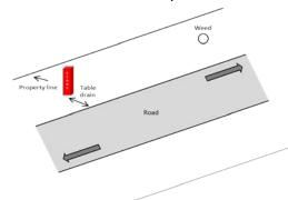
Location along roads with no existing guide posts: Red guide posts are to be installed the fence side of the table drain so as not to hinder grading. Note: grader operators should be checking with the weed officer prior to entering a red guide posted site.
